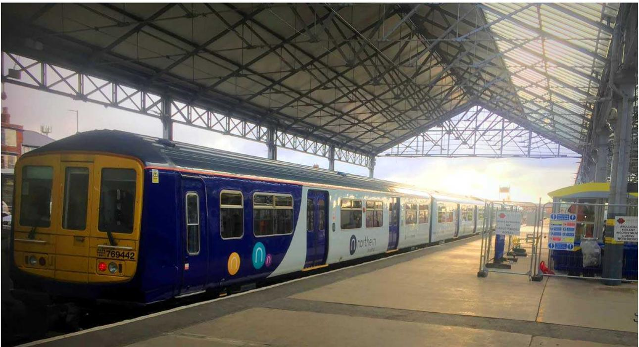
Finally, a picture of a full size, 12 inches to the foot scale train. This shows 769 442, one of the new tri power (25Kv AC, 750v DC and diesel electric) trains, formerly a Thames Link Class 319 dual voltage electric unit, in Platform 6 of Southport Station alongside the new passenger shelter which is being erected. I thought it was on driver training but in fact it had broken down and was awaiting attention and eventually limped back to Springs Branch! **Jim Ford.**
