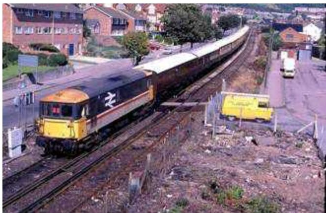
The British train was usually hauled from London Victoria to Folkestone East by a Class 73 electro diesel. As a reversal of direction was required, a Class 33 diesel electric was attached to the rear of the train and a cautious descent was made to Folkestone Harbour. Whilst the passengers alighted, both locos changed ends ready for the return working to London. On departure, the Class 33 would lead and the Class 73 push for
