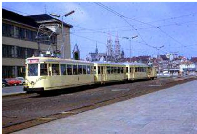
The connotation Interurban Railway may be a term not familiar to some but to explain, an Interurban Railway could best be described as a fusion between a street tramway and a full sized railway. The generally larger Interurban cars would share street tracks with the streetcars (or trams) and on reaching city limits entered their own trackage where greater speeds could then be achieved on their own private right of way.
