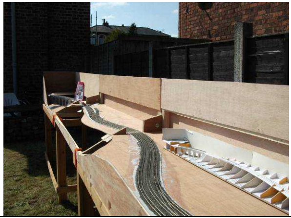
Views showing effect of thermal expansion on track geometry. Only the middle board was impacted and was caused by an extra 1mm expansion on 1500mm of track constrained at either end.
