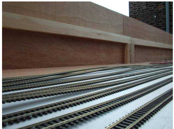
Views showing effect of thermal expansion on track geometry. Only the middle board was impacted and was caused by an extra 1mm expansion on 1500mm of track constrained at either end.
