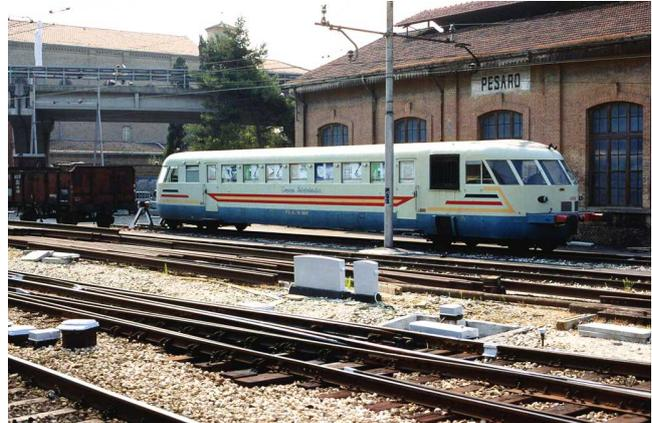
Starting from 1938 to 1940 some FS passenger railcars of type ALn 556 and ALn56, built by Breda, started running on the Italian lines, thus introducing an evolution in the railway traffic. ALn56 were so classified since, contrarily to ALn556 they hadn't the double heading devices under multiple unit control (two railcars driven by a single driver).
