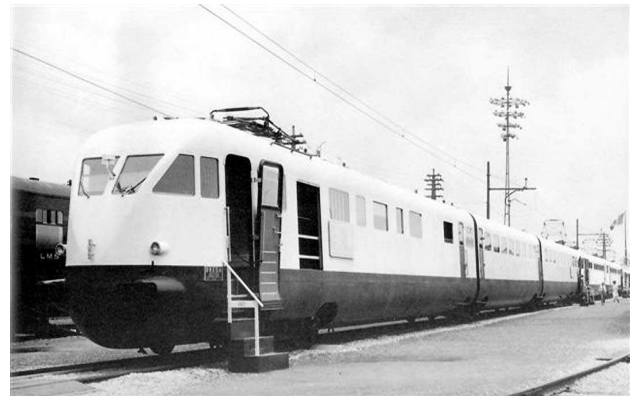
Captions. The picture on the left shows an ETR200 three car articulated train in service on Italian State Railways. The picture on the right shows an ETR200 train on static display at the 1939 New York World Fair. Note the authentic Italian style overhead electrification. Also, the astute observer will notice an example of LMS coaching stock in the background.
