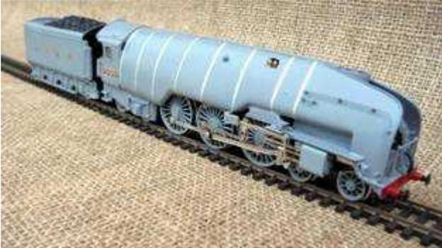
The LNER W1 No. 10000 (also known as the Hush-Hush due to its secrecy and Galloping Sausage before rebuild due to its shape) was an experimental 4-6-4 four cylinder compound steam locomotive fitted with a high pressure water tube boiler. Nigel Gresley was impressed by the results of using high pressure steam in marine applications and so in 1924 he approached Harold Yarrow of shipyard &
