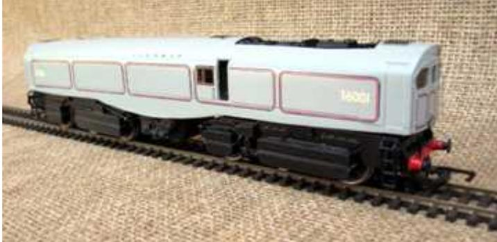
The Southern Railway Leader was a class of experimental 0-6-6-0T (C-C) six cylinder articulated steam locomotive, produced to the design of the innovative engineer Oliver Bulleid. The Leader was an attempt to extend the life of steam traction by eliminating many of the operational drawbacks associated with existing steam locomotives. It
