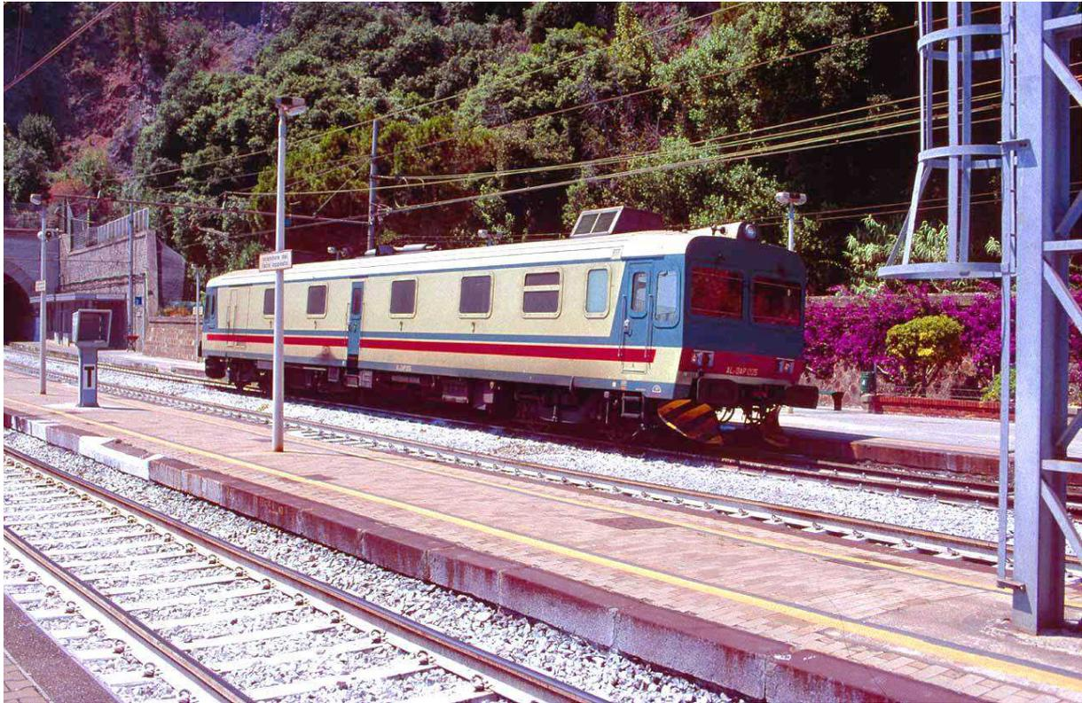
The self propelled railcars are built by FIAT Ferrovia in a style closely resembling that of their ALn 663 passenger diesel railcars. To explain the class designation, the A is for Automotrice (Automotor), the L is for Leggero (Lightweight) and the n is for Nafta (diesel fuel). The 663 indicates 63 seats with the repeated first number indicating that the vehicle may be operated in multiple with other railcars.
