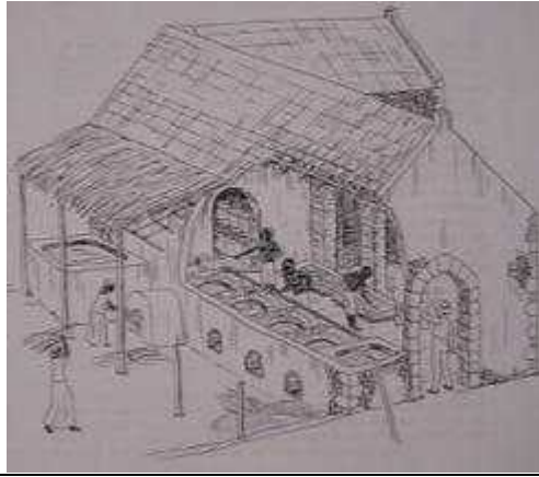
Boiling room with series of kettles, "refined" sugar is ladled from one to the next one to improve clarity
